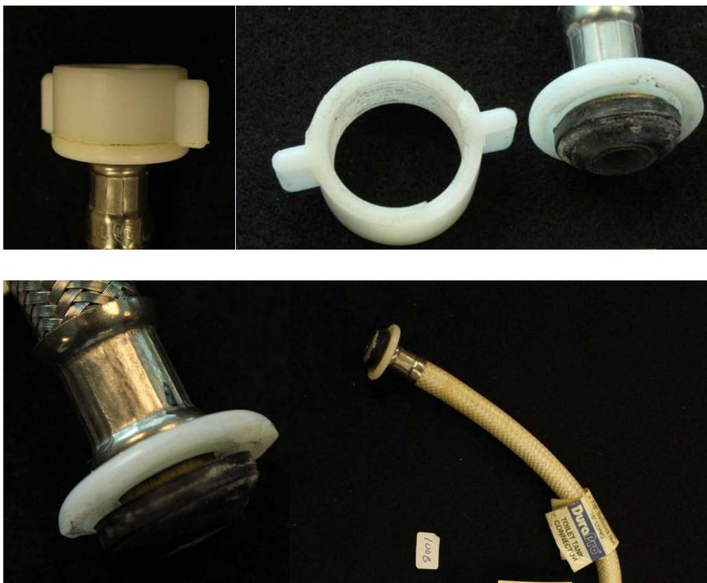
47. These repeated spontaneous circumferential fractures are the direct result of the inferior design and materials used for the Toilet Connector which led to a uniform defect in all Toilet Connectors. The Toilet Connector's plastic coupling nut failed to adhere to the most basic
